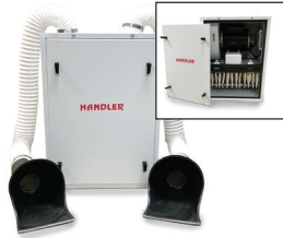
60U-D - Dust collector with clean-out tray, two 4' sections of 3" flexi-hose, two fishmouth suction inlets, four metal clamps, 14 sateen cotton-cloth filter bags, and easy-to-use foot pedal to shake out and clean bags.
