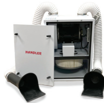
60UFC - Dust collector with clean-out tray, two 4' sections of 3" flexi-hose, two fishmouth suction inlets, four metal clamps, and one state-of-the-art pleated drum cartridge filter.
